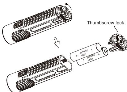
**NOTE:** After battery insertion, the power indicator light will blink to indicate remaining battery power. Please refer to the "Power Tips" section of this manual for details.
